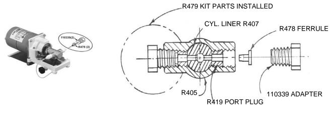
CROSS-SECTION VIEW OF STANDARD STAINLESS- STEEL CYLINDER CASE ASSEMBLY AS ADAPTED FOR LOW FLOW, LOW DEAD VOLUME APPLICATIONS
